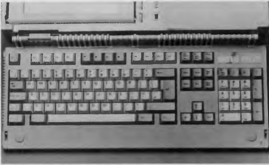
Figure 3. The keyboard is a standard AT style layout with separate cursor control keys, numeric pad and 12 function keys. The right hand Alt key is used in conjunction with Scroll Lock to switch between the LCD screen and an external monitor.
