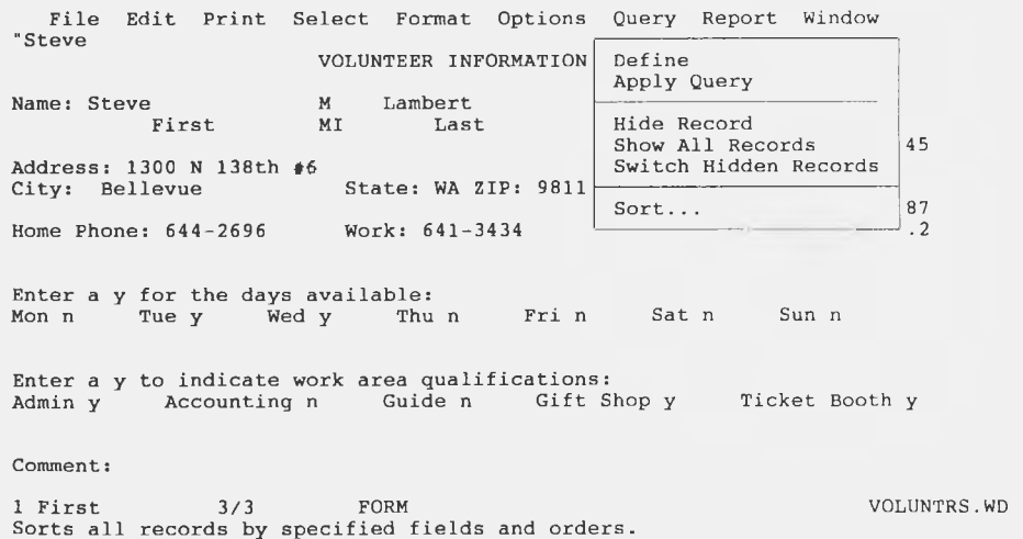
Figure 2. The RAM based Works database offers two views of the data – List shows one line per record and one field per column with several records onscreen at once, while Form (shown here) shows one record at a time for updating.
