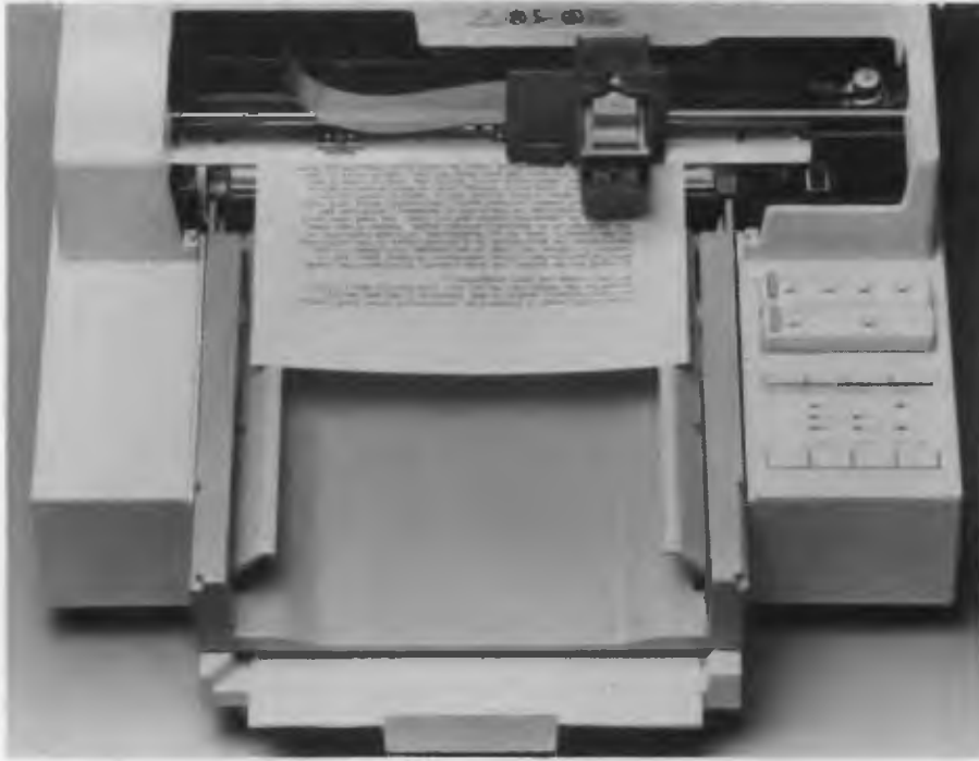
Figure 6. The self-cleaning, self-parking head of the DeskJet is suspended vertically above the paper as it prints. Note the two rails supporting the freshly printed page as it emerges.
