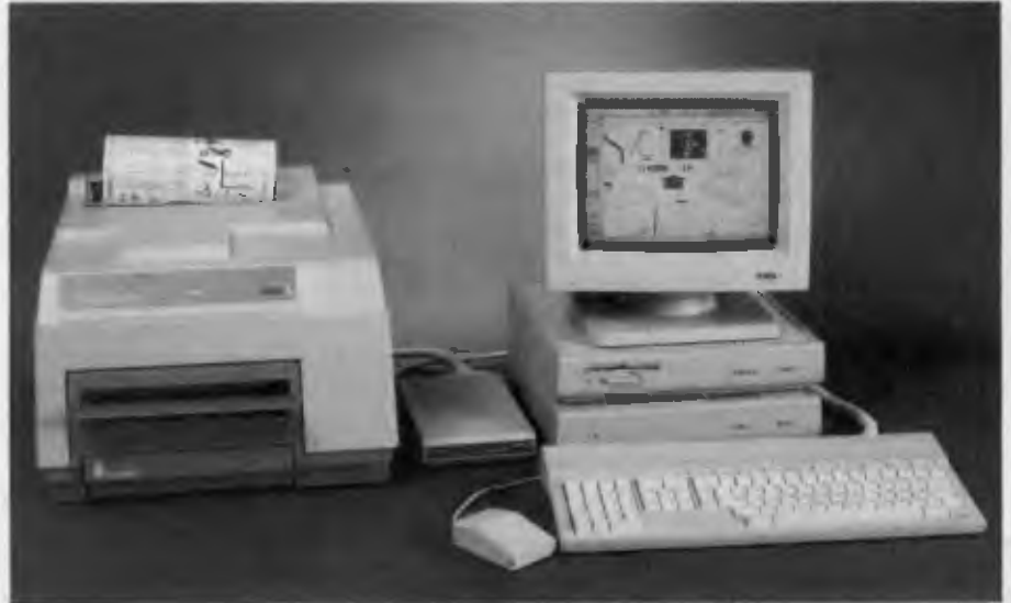
Figure 1. The two models of the Mega ST, the Mega 2 and Mega 4, both feature a DMA port for connection of a hard disk unit or laser printer.
