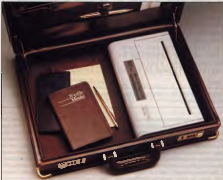
Figure 4. Kodak's Diconix 150 Portable – this innovative 12-jet machine runs from batteries stored in the platen.
