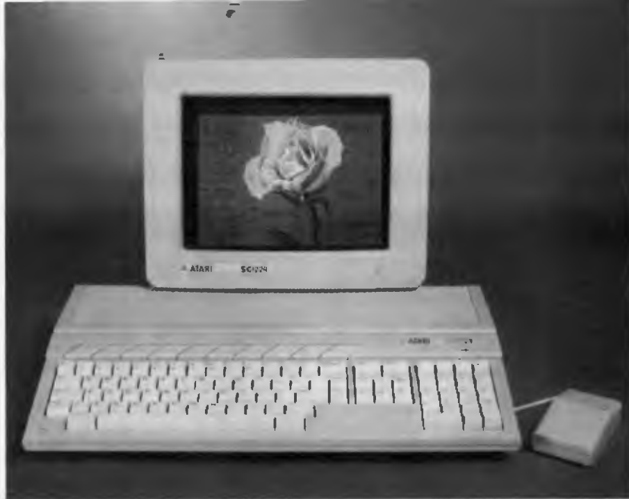
Figure 2. The 520ST has 512 Kbyte RAM, 360 Kbyte disk storage, 512 colours, a 68000 processor running at 8 MHz and a MIDI (Musical Instrument Digital Interface) port.
